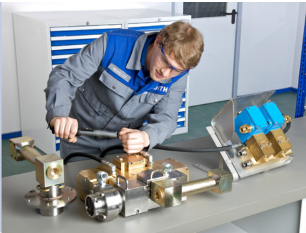
Control block STB7/300 F: Customer-specific solution for filling and emptying a fill-controlled fluid coupling using a fresh-water or pneumatically-controlled pilot unit
